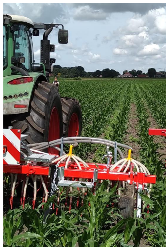
Mechanical weed control: hoe with camera control and GPS-supported section control and intensive harrow
